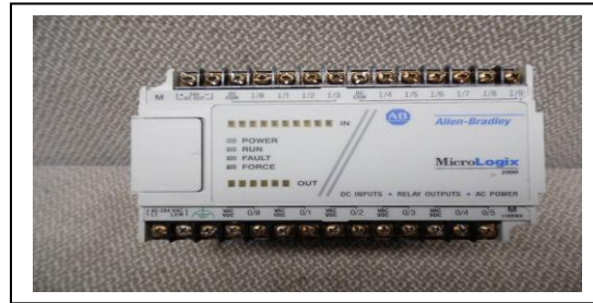
Figure 4: A 16I/O Allen-Bradley PLC
